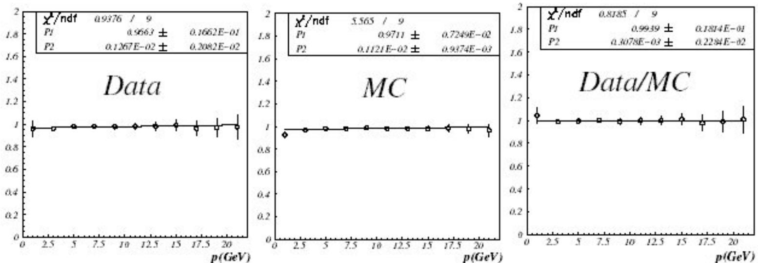
For tracks hitting all superlayers, the average efficiency in the full kinematical range is  $(96.7 \pm 0.9)\%$  and it is almost constant.
