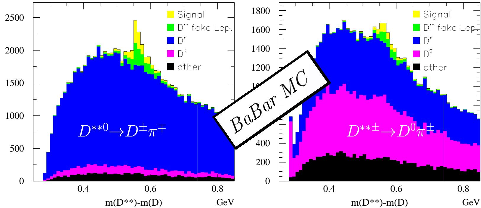
Signals are defined in the mass-difference  $\Delta m = m(D_{rec}^{**}) - m(D_{rec}^0)$ , this improves the resolution since systematics cancel out.
