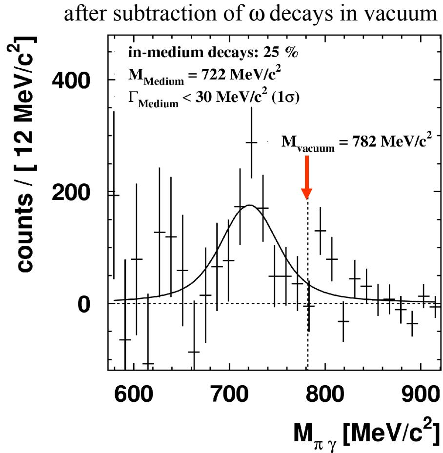
$\omega$  in-medium mass:  $720^{+35}_{-5} \text{ MeV}/c^2$  consistent with  $m_\omega = m_0 (1 - 0.14 \rho/\rho_0)$
