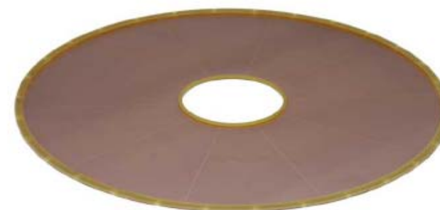
Mounted GEM Foil on Frames
