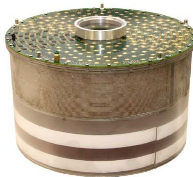
Prototype TPC with 10cm drift depth
